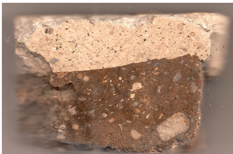
Fig. 1 Polished earth and lime plaster sample, York House, Malton, showing both quicklime and oolitic limestone content in the lime finish coat of lime and hair only, with naturally present aggregate within the burned limestone.
