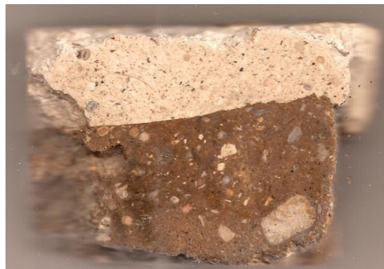
Figure 6 : polished earth and lime plaster sample, York House, Malton, showing both quicklime and oolitic limestone content, lime finish coat of lime and hair only, with naturally present aggregate within the burned limestone (Gourley)
