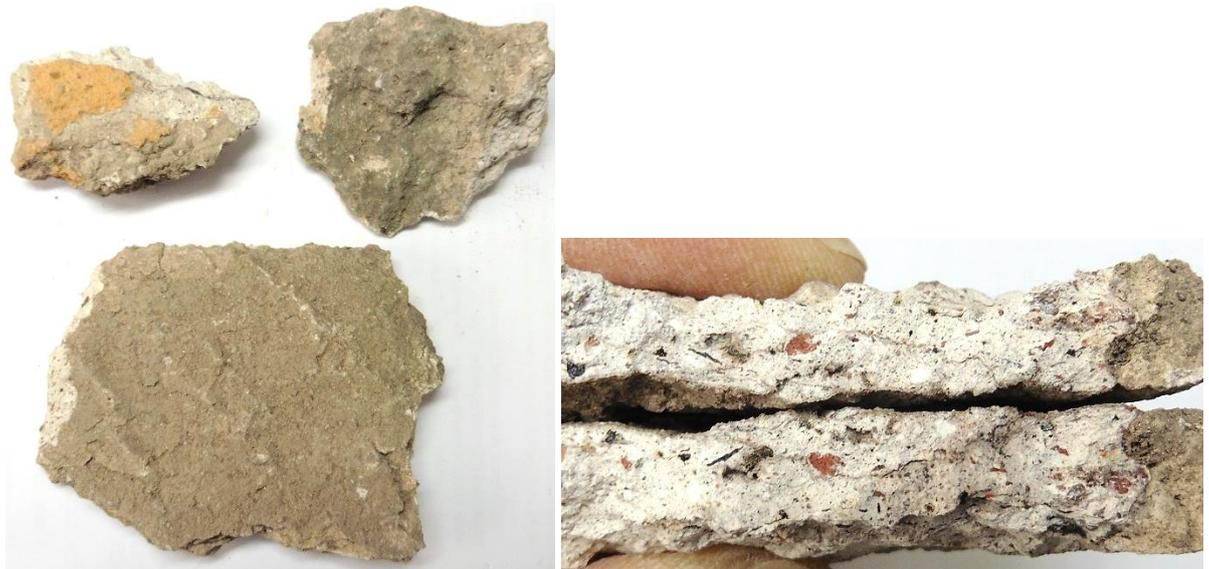
**Plates No. 3 & 4:** The left plate shows the three pieces in the sample received. These all displayed one face that was heavily soiled, with the soiling locally encapsulated with a coating of redeposited calcite. The right plate shows a freshly fractured surface through the thickness of the larger intact fragment, note the presence of an abundance of lime inclusions, with dark slag fragments and red brick fragments distributed throughout the mortar.
