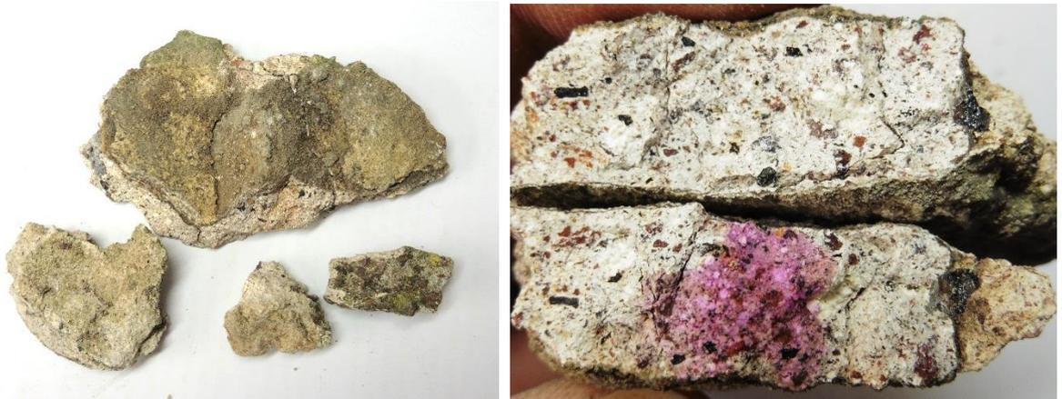
**Plates No. 7 & 8:** The left plate shows the intact pieces of mortar in the sample received. With the right plate showing a close-up of a fractured surface, through the largest intact piece, where the dense condition of the fabric is seen, along with an abundant of lime inclusions. The lower fragment is shown after testing with a phenolphthalein indicator, note pink colour.
