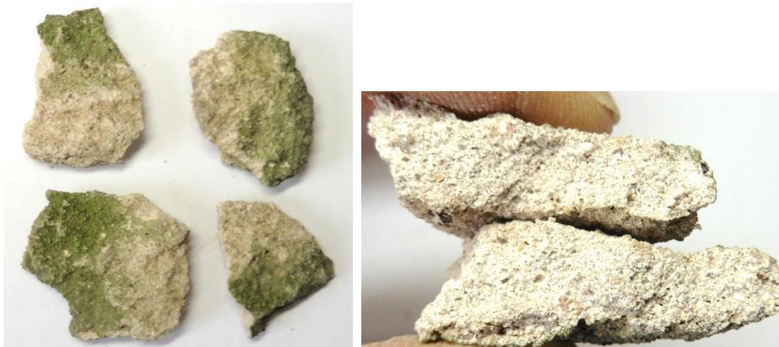
**Plates No. 1 & 2:** The left plate shows the intact pieces of mortar in the sample, as received, with the right plate showing a magnified image of a freshly fractured surface through the thickness of the sample. It was noted that the lime inclusions observed were small and randomly distributed throughout.
