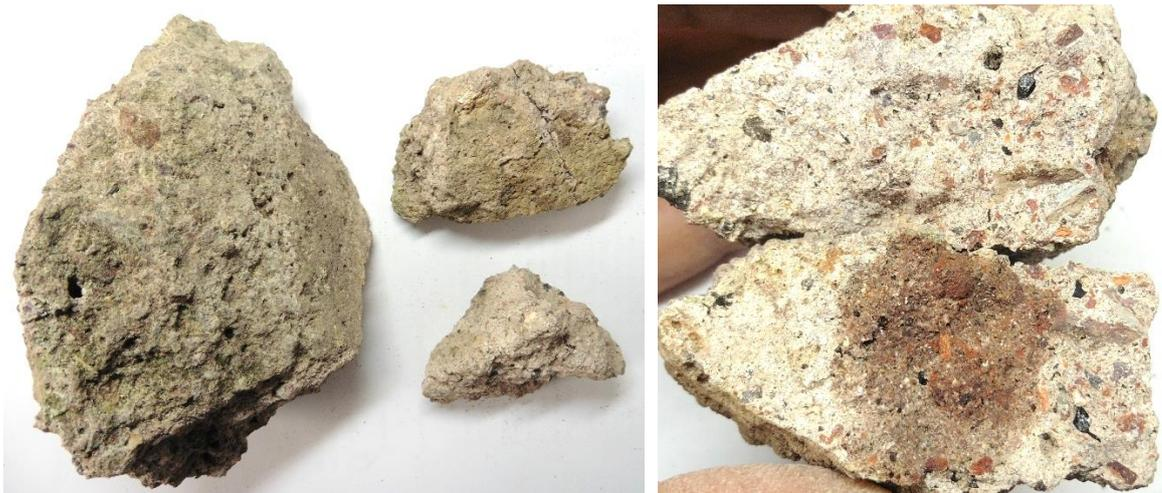
**Plates No. 5 & 6:** The left plate shows the three intact pieces of mortar in the sample, as received. The right plate shows a close-up of a freshly fractured surface, where the dense condition of the fabric can be seen. Note the abundance of small white lime inclusions, randomly distributed throughout. The lower piece is discoloured where it had been tested with the phenolphthalein indicator solution, with no colour observed in the paste, suggesting that the mortar was fully carbonated.
