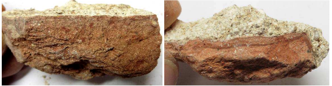
Plates No. 3 & 4: Both of the above show examples of the mortar adhering to pieces of the brick, which was typical of all of the pieces received.
