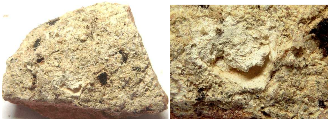
Plates No. 5 & 6: The left plate shows a view of the surface of the mortar adhering to the brick fragment in Plate No. 4 above. This being the thickest depth of mortar on any of the pieces received was used for thin section preparation. The right plate shows a close-up of one of the large lime inclusions observed in the mortar.
