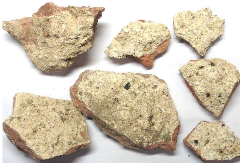
Plate No. 1: The above shows the sample as received with the mortar coated face of the brick fragments shown. The inner surfaces were of fractured soft brick and are shown below.
