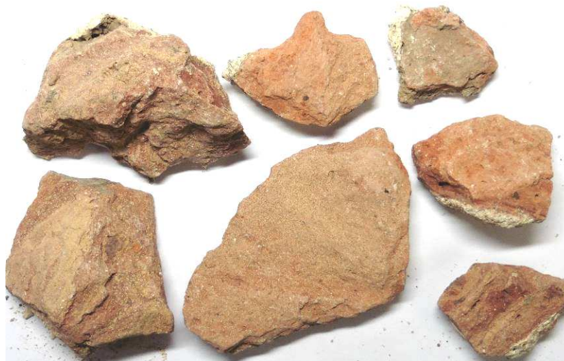
Plate No. 2: The fractured, mortar free surfaces, of the brick pieces are shown above.
