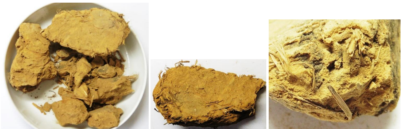
Plates No. 8, 9 & 10: The left plate shows the sample as received, with the centre image showing an intact piece of plaster, with straw well bound within the clay, with the right plate showing a magnified image of a freshly fractured surface to show the density of straw fibre within the plaster.
