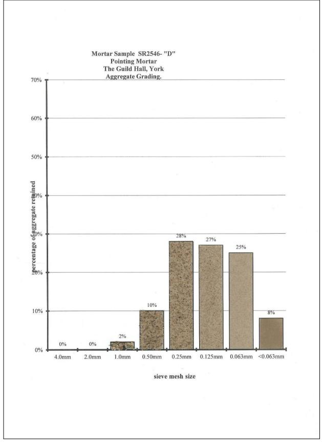
Figure No. 1: Grading of Aggregate from sample SR2546-S3 "D"
