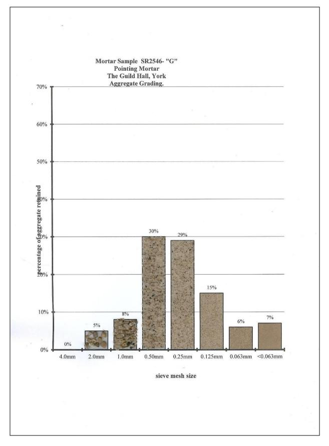
Figure No. 3: Grading of Aggregate from sample SR2546-S6 "G"
