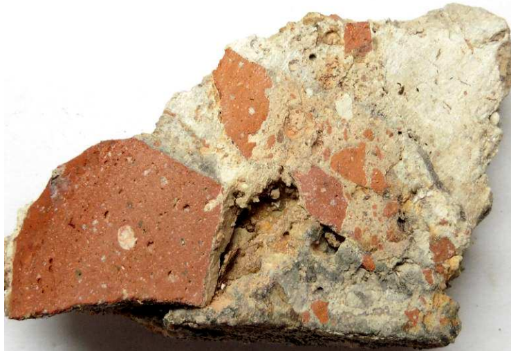
Plates No. 1 & 2: The above plates show the condition of the sample as received in the laboratory, with the left plate showing the outer surface of the mortar, which retained algae and moss adhering to its surface and penetrating into surface connected voids. The presence of the organic growths and surface soiling inferring that this mortar sample was removed from a section of masonry exposed at the surface. The right plate shows the inner masonry contact surface, where large tile/brick fragments along with a large limestone fragment appear to form the main aggregate components.
