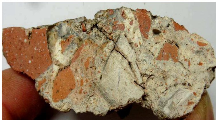
Plate No. 4: The image on the left shows the piece of the mortar from which the petrographic thin section was prepared.
