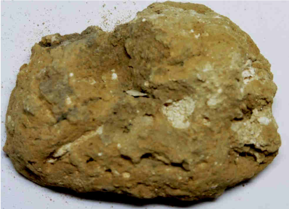
Plate No. 1: The above shows the outer surface of the sample as received, prior to drying. Note the high abundance of lime inclusions, the inclusions mostly have rounded margins and from the initial examination it is indicated that the lime was probably used in the form of a putty lime, width = 64mm.
