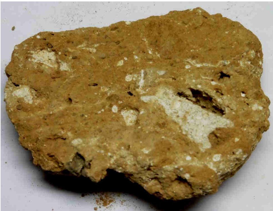
Plate No. 2: This shows the sawn surface through the plaster, from which a slice was removed for the preparation of a petrographic thin section. Note that the mortar is lime rich. Width of sample = 60mm.
